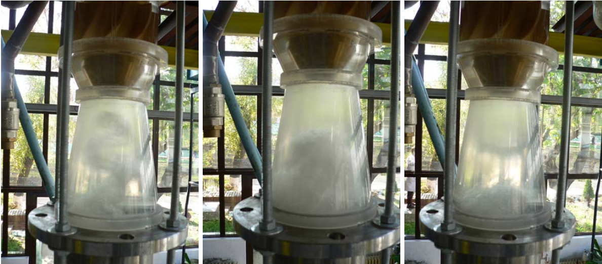
a) no jet control b) with axial control jet discharge at two different values
